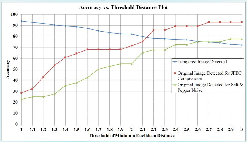
Detection Accuracy vs. Threshold Distance plot
